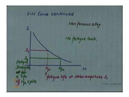
But a different kind of behavior is seen in some non ferrous material. Non ferrous alloys where there is no fatigue limit in this case.
