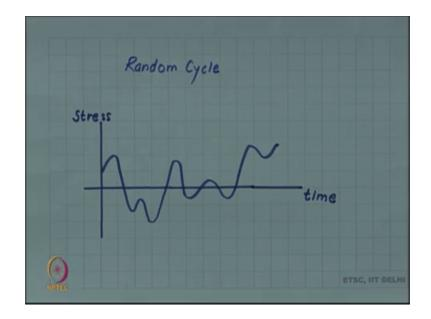
This is also important, this is the failure in cyclic loading is at a stress considerably lower than yield stress.
