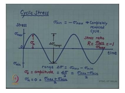
Let us look at what a cyclic stress means. Here we have a nice symmetric completely reversed cyclic loading. In which the stress varies from 0 to a maximum tensile stress sigma max and then comes down, to a minimum stress which is a compressive stress and has the same value in magnitude as sigma max.
