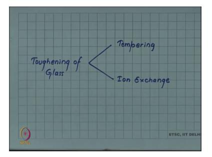
We have already considered the process of tempering which is a physical process for toughening of the glass; ion exchange is a chemical process.
