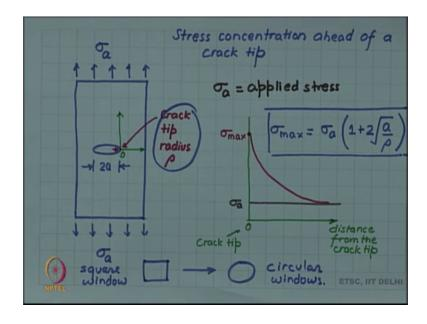
So, this is a crack in a body under an applied stress of sigma a. So, sigma a is the applied stress but if we look at the stress along this line starting from the crack tip and going away from that along this line and plot the stress on the y axis, let us do that. So, origin is at the crack tip and this is distance from the crack tip, then what you find is that if and let us say that this stress let me plot.
