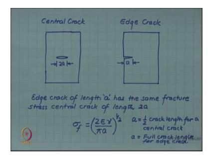
In the Griffith plate which we analyzed the crack of length 2a, was in the centre of the plate but the paper experiment which I did was with edge cracks. So, how the 2 situations compare? It turns out that actually edge cracks are more dangerous because edge cracks of length a has the same fracture stress at central crack of length 2a.
