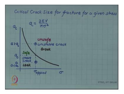
If we plot this curve, if we plot this curve a c as a function of sigma you can see with increasing sigma it will keep decreasing. So, you have you have a curve like this. How do we interpret this curve?
