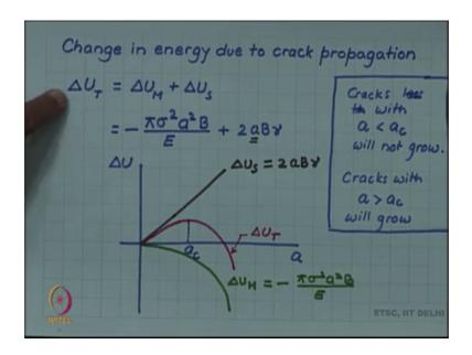
So, now, I have two component of energy change in the system that is a the mechanical energy change delta U M, and the surface energy change delta U S, we saw that we did not derive but we saw that the delta U M can be written as minus pi sigma square a square B by E whereas, the surface energy can be written as 2aB gamma.
