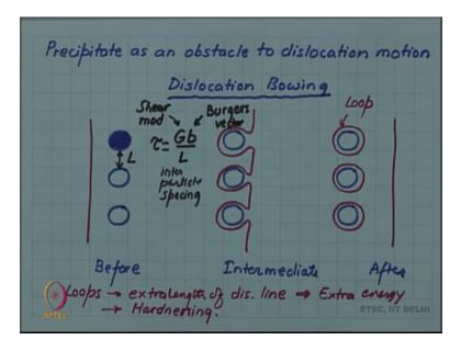
When the precipitates have become much larger towards the later part of the hardening and during over aging, the precipitates become too large to be cut; so, it is not easy to cut these precipitates, but the spacing between them is large enough recall that by Ostwald ripening, the spacing is becoming larger and larger. So, a spacing between them become large enough such that the dislocation can bow between them.
