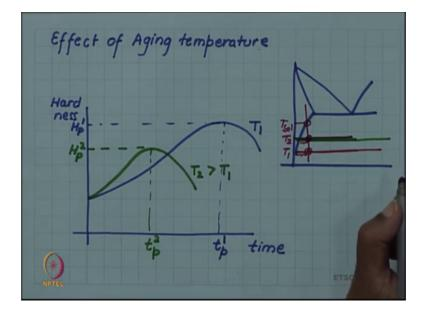
So, now more or less we have seen the explanation for the aging curve. Initially as more and more precipitates form, more and more obstacle to dislocation motion is there. Finally, when all the precipitates have formed we have a fine distribution of precipitate fine and numerous precipitates are there.
