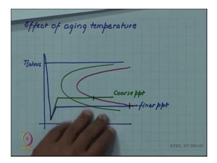
So, suppose you quench and then you aged at this temperature or you aged at a higher temperature. We have already seen that at the higher temperature, you will have coarser precipitate because of slower nucleation and faster growth whereas at a lower temperature you have finer precipitate. So, this fine precipitate will give you a higher hardness.
