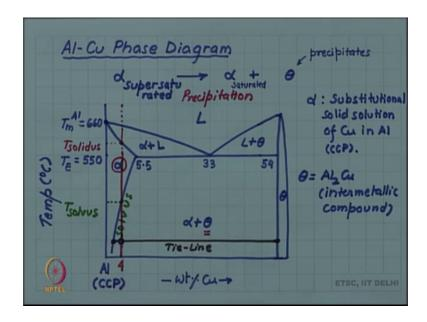
First of all look at the aluminium copper phase diagram; it is very important when discussing any alloy to look at its phase diagram. So, in an aluminium copper phase diagram, this left axis is the aluminium alloy, sorry, pure aluminium axis and the melting point of aluminium 660 degree Celsius is listed there, this is the temperature axis as you are now well familiar with a phase diagram.
