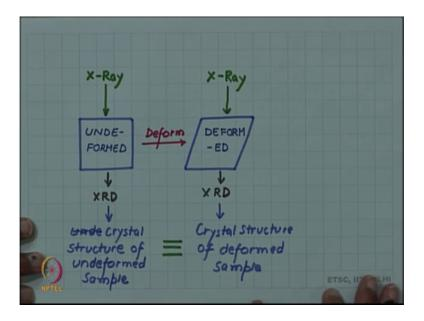
So, let us subject our undeformed and deformed material both of them to X ray diffraction. So, I sign X ray on undeformed material and I also sign and then I deform it. And I do the experiment again I sign X ray on the deformed sample both will give me the fraction pattern the X ray diffraction. And when we analyzed the diffraction pattern we can solve the structure and we can find, what has happened to the structure.
