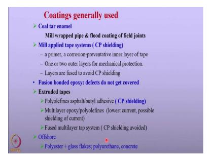
The listed one on the top the coal tar enamel is one of the oldest coatings applied on the pipeline. Nowadays, it is being reduced or in some countries they are they are almost eliminated and these coatings are applied using mill wrapped the pipe on the on the shop floor or on the field you use a flood coatings the molten coal tar enamel is applied over the field joints.
