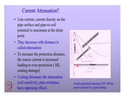
This is related to current attenuation that occurs in the pipeline. Let me now describe what is current attenuation. What is shown in this diagram on the right side of the slide is the variation of the potential and the current with respect to the distance across the pipeline from an anode location. Now, what you notice here is that the both the current and the potential is maximum at the pipeline in the vicinity of the anode location.
