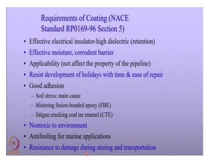
So, now we understand that coating is very important and it indeed is complementary to cathodic protection of structures, then we should look at what are the requirements of a coating that will make the cathodic protection very effective.
