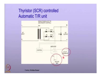
What I shown here is a schematic of a thyristor control automatic TR unit. The two important things that you look at it one is pipe to soil potentials this is measured using a reference set reference here right. So, if the pipe to soil potential is changing because of various conditions as we talked about before say stray current or coating defect has happened or because of the climatic conditions you know wet conditions happening.
