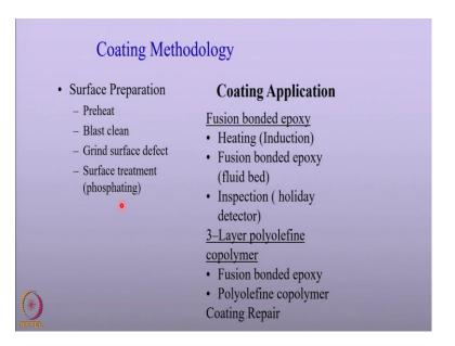
Let us move on to the coating methodology how these coatings are applied. We all know that the performance of the coatings against corrosion depends upon the quality of the coatings. We talked about you should have high electrical resistance high dielectric constant, but it is not sufficient to have a good coating, it is also important to apply this coatings properly an improper application of the coating does not give better performance. So, that starts with surface preparation.
