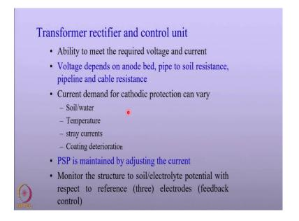
We shall now move on to the next topic of discussion today that is Transformer Rectifier and Control unit this is called as TRU in the cathodic protection parlance. The rectifier must able to meet the required voltage and the current for cathodic protection of the intended structures.
