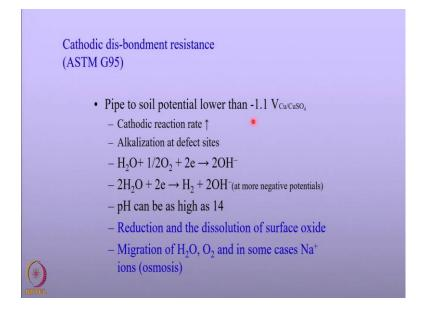
As we have seen earlier in few of the lectures that when the pipelines or the structures are protected using ICCP that is Impressed Current Cathodic Protection systems and its very likely that at some regions of the structures the potentials go well above the required potential criteria that is - 0.85 volts with respect to copper sulfate.
