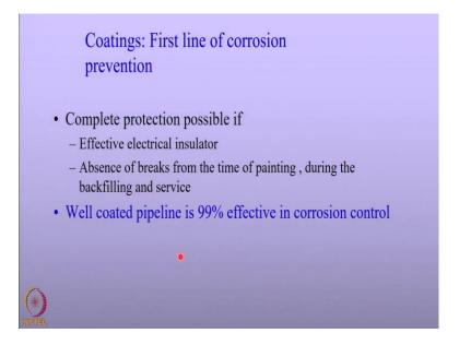
First one would ask the question, why would someone to coat a pipeline or a structure if these are cathodically protected? On the other hand, if someone coats in the structure with a protective coating, why would one would go for cathodic protection?
