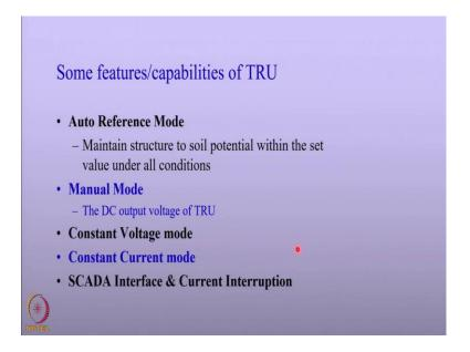
Some other features and capabilities of TRU as you seen before it is auto referencing mode it maintains the pipe to soil potentials all through the rectifier must also have the capacity to operate using a manual mode to change the dc output in terms of voltage or maybe in terms of current also.
