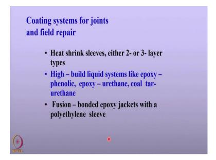
We have seen so, far coatings applied at the mill the coatings are also applied on the field one is for the joint joints and other whenever the coating is damaged. The three types of coatings are applied in the field it could be heat shrink sleeves either of 3 or 2 layer types like what is in polyethylene the polypropylene type or it could be epoxy phenolic epoxy urethane coal tar urethane and so, on so, forth.
