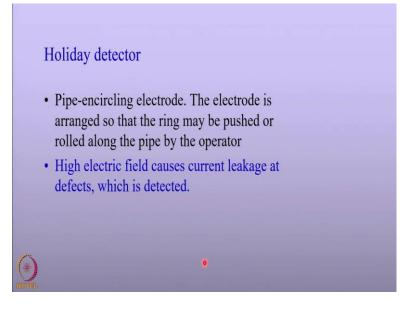
We know that the holidays in the coatings could be detrimental, it can lead to cathodic disbondment, it can lead to higher current demand. So, it is important to inspect the pipeline against the presence of holidays.
