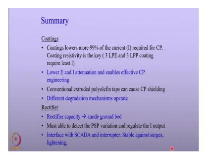
We looked at the two important topics of cathodic protection one is coatings other is rectifier. We saw that coatings and cathodic protections are complementary. Coatings make the cathodic protection very efficient it also reduces the current demand for cathodic protection and there are different types of coatings among them three-layer polyethylene coatings, three layer polypropylene coatings are considered to be most effective in reducing the current requirement for cathodic protection.
