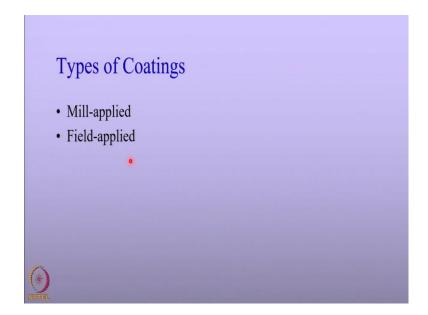
Let us come to the coatings, we have two types of coatings depending upon the applications one is mill applied that is applied in the shop floor and the pipelines are pre coated actually and then transported to the site, the other kind of coatings is the field applied coatings because even the mill applied coatings or pre coated pipelines there are certain edges of the pipeline, it is not being coated because they need to be welded.
