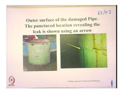
You see it is a pipeline and in fact, this pipeline carries water from the chiller and goes to the heat exchanger and you know. In fact, it is it was used for one of the five star hotel where the air conditioned system. You know you know the air conditioned systems how it works. And you see this is this pipeline is carrying the cooling water.
