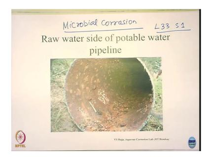
Welcome to the next chapter on the Forms of corrosion. And today we shall be discussing on what is called as Microbial corrosion. What I have shown here it is a pipeline got corroded due to microbial corrosion. To be more specific; the presence of sulfate reducing bacteria and the iron bacteria were implicated in the corrosion of this particular pipeline.
