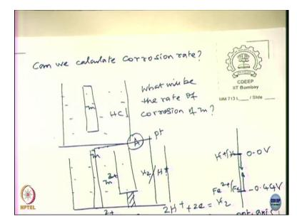
Now, comes can we calculate can we calculate corrosion rate? Say, I have immersed Zn in let us say hydrochloric acid. You know how to compute whether it corrodes or not rather corrodes or not use the Nernst equation. Now, in Zn in hydrochloric acid what will
