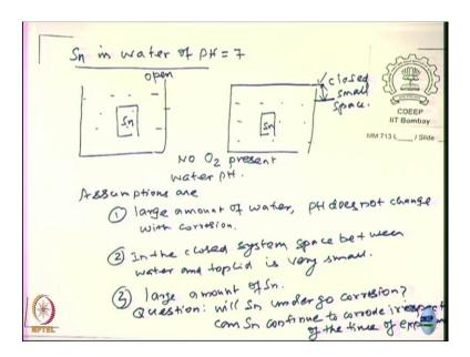
The problem is I take Sn in water of pH 7 ok. Two conditions take water and immersed in here in another case I take water I have Sn, I close this here; this is open ok. This what about here in this case? Is closed, no oxygen present, no oxygen present and the water of pH is about 7. So, the pH of the water here you know the water pH is 7.
