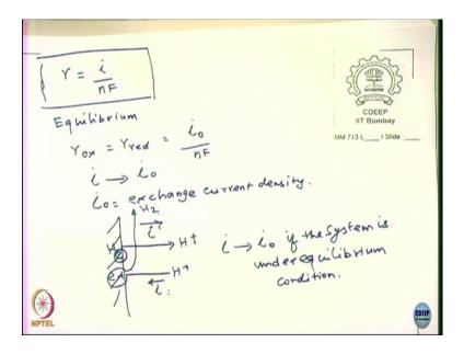
Yeah, now we have seen now the rate of reaction r = i / nF. Under equilibrium what happens? The rate of oxidation is equal to rate of reduction then what happens? Then and what happens now  $i_0 / nF$  that means, i tends to become  $i_0$ . What is  $i_0$ ?  $i_0$  is defined as exchange current density ok.
