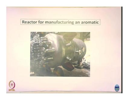
This in fact, is an ongoing work which we have been do we are doing now. This is the reactor, in fact is a pressure vessel I would say. It is high pressure. It is meant to produce an aromatic compound you know most of you know the aromatic compounds are you know as a special characteristics. And they are synthesized using inputs which are mostly organic and may be some time, you may add sodium hydroxide, you need water. You are subjected to high temperature, high pressure conditions.
