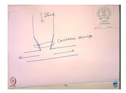
Suppose, I have a pipeline like this, they were to join onto this pipe actually. They reduced like this. Now, look at this design here is a pipe, the larger diameter, smaller diameter, you welder like this.
