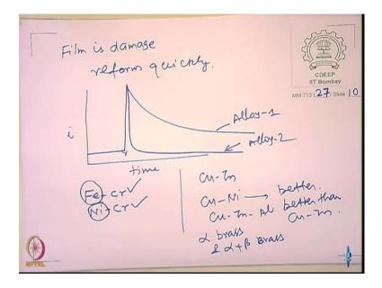
This is the passive current, if I damage here, current will rise, it can go like that or it can go like this alloy one, this is going to be your alloy two, which is better, alloy two is better. So, the alloy development program will take care of both the electrochemical and the metallurgical aspect of corrosion.
