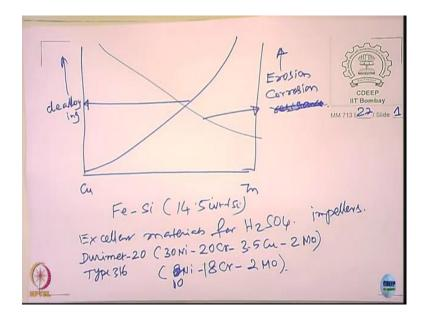
The limited extent, de alloying erosion corrosion resistance. No, I do not all resistance here, I say erosion corrosion both scales are going same manner, ok. Can you plot how this will happen?
