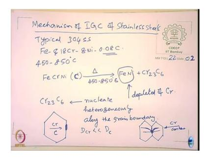
Actually, now you can refer that as well. Let us now discuss about the mechanism of IGC of stainless steels. Please notice that the mechanism of IGC of stainless steels is not same as the mechanism of intergranular corrosion of other kinds of alloys actually. So, you cannot just generalize this mechanism everywhere and we see that as an example for aluminum alloys.
