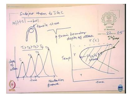
Maybe you can take a hydrochloric acid HCl you can take some maybe you know 10% HCl you can take and boil that, expose the sample. And take the sample out in this case and you can bend the sample over a mandrel you can bend it over mandrel.
