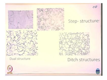
So, it suffers intergranular corrosion. What it is? I have shown you the micrographs of stainless steel under different conditions of treatment. The top one you see here is, see the low magnification of this, this essentially is a mill annealed kind of situation where they heated to 1050  $^{\circ}$ C and then, quenched in water and then, they carry out a test they called ASTM A262 a test we will see later to reveal the grains here.
