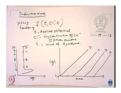
Actually, just to make some remarks, I would say pitting corrosion, pitting tendency is a function of applied potentials, the chloride or anion concentration. Then, the time is going to be other factors. E, where here E is applied potential, chloride is the here concentration of chloride or other anions, time is the time of exposure.
