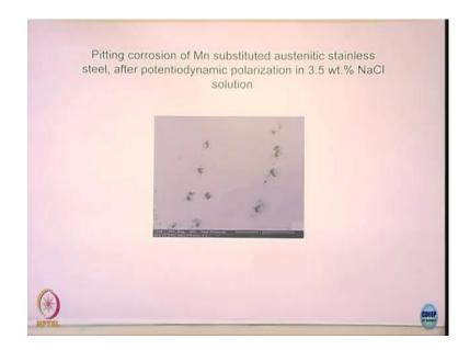
And they can start damaging. Sometimes the pit also can have a very complex morphologies, will see later actually. You can see here these pits, these are all corresponding to a stainless steel, where nickel was substituted with the manganese and why is people substitute nickel with the manganese? Because the manganese is cheaper and also, you can stabilize the austenitic phase.
