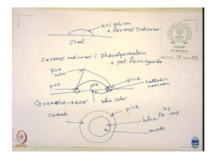
In another case you can take a steel take a steel and you have a drop of potassium chloride solution right you have a drop of potassium chloride solution with water. And to this you add what is called as ferroxyl indicator add to this and what is a ferroxyl indicator?
