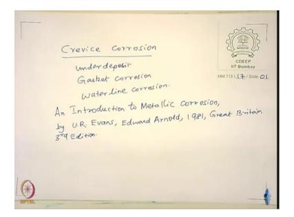
So, crevice corrosion is a common name. So, it is called as also as under deposit. Some time called as gasket corrosion and is of course, similar to that is called as waterline corrosion. In all these cases there is something very common. It is a common mechanism. This particular type of corrosion problem is industrially very important ok.
