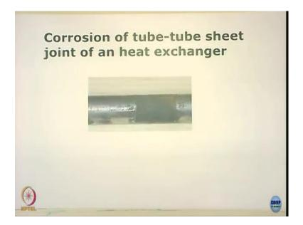
So, these are the typical you call gasket corrosion or crevice corrosion joint corrosion problem. You have the other kind of joint you will see in the case of a the heat exchanger we probably brought out this heat exchanger in one of the previous classes.
