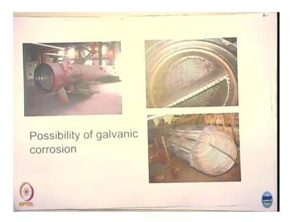
This is done mostly in industries I just given, this figure you seen before right and it is an heat exchanger, this is the this is called as header or water wall boxes header it is; these tubes generally are stainless steels, that the galvanic corrosion here. How do I control galvanic corrosions?
