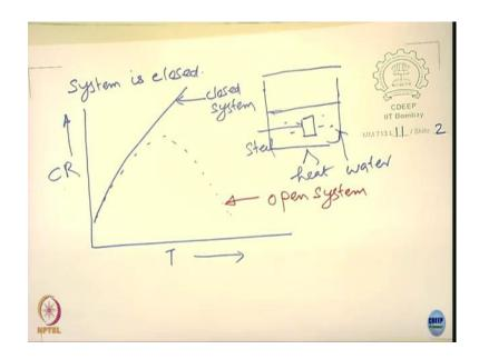
The system is closed not you know open to the atmosphere ok. Say, we have a beaker and I just close it here and I have water up to this levels, have a steel and this is water this is steel and it going to heat it now ok. So, what do you think will happen in this case? What will happen to corrosion rate with temperatures? Yeah.
