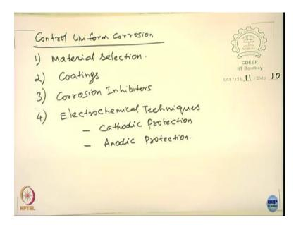
So, how do we control uniform corrosion? 1, I can choose a proper material selection you can do that you can also look at the coatings. We can also see the use of corrosion inhibitors and 4; we can also use electrochemical techniques. What I mean by this? Here you can use or employ cathodic protection we can also employ anodic protection.
