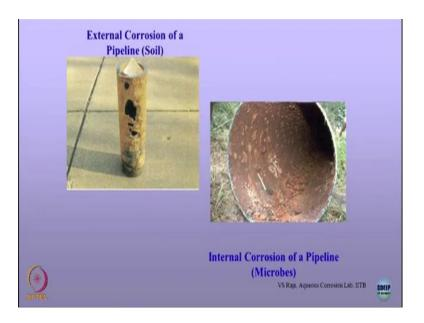
I given this example, pipeline I think some of you would have seen it, here this is internal this is external corrosion entirely different. The internal corrosion depends on what? Depends upon the water chemistry water it is going to use.
