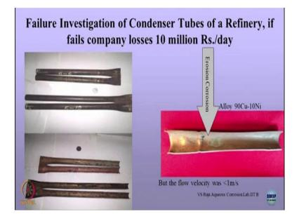
Very similar issue, this is refinery is again close to us, a simple condenser tube in a refinery they were using seawater. Seawater you cannot use carbon steel you know because of high velocity it is a problem you cannot use stainless steels, they start using copper nickel alloy it is called cupro nickel alloy right alloy.
