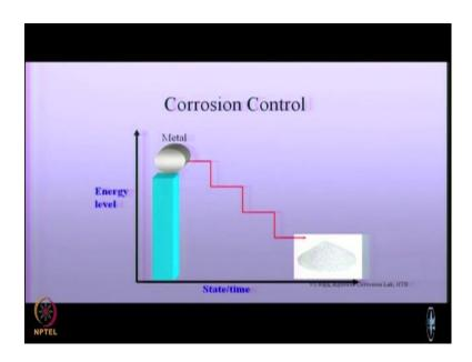
Now, as you have seen before thermodynamically, most of the engineering alloys the structural materials are bound to corrode right. Why? Because the energy of the metal is higher and any time it can form it can corrode. Can you ever completely stop from corrosion? You cannot forever you cannot forever cannot stop it what we can do is, we can slow down the corrosion process right.
