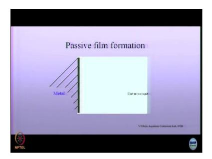
You have metal here; it comes in contact with environment here what it has to do? It forms a film on the surface and this film is a barrier for the environment to come in contact with. This is corrosion stainless steel all of us know. Can you give another example of a reactive material having high corrosion resistance? Yeah?
