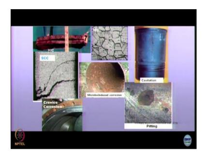
We have seen this before. this is called hydrogen induced cracking, hydrogen gets into the material and then builds pressure and cracks. This is called stress corrosion cracking when you apply a stress and you have environment it cracks, you know when it cracks its brittle what is the ductility of a typical 316 alloy stainless steel. Anybody here can tell? Ductility is could be 60 percent ductility; it spread that is why metals are used.
