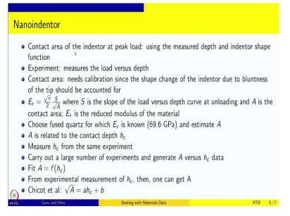
So the contact area of the indentor at peak load that we want to get using measured depth and the indentor shape function. So the depth measurement is made and we know what the indentor is, but sometimes the experiment is load versus depth, so we will know the load, we will know the depth and that is from where we are getting the depth.
