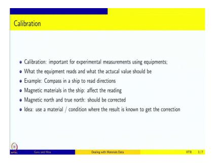
Calibration is important for experimental measurements using equipment and what the equipment reads and what the actual value should be, there could be sometimes discrepancies. The very well-known example that is also described in Berenson's textbook, for example, is compass reading in a ship to read directions, because there are a lots of magnetic materials in ship that affects the reading.
