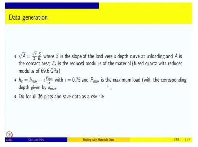
There is a relationship. So we already know this, so root A is root pi by 2 S by Er,, so pi by 4 S squared by Er squared is actually giving you the A because we know the Er and we can measure the slope from the this curve. So this is basically the slope of this red line you see here.
