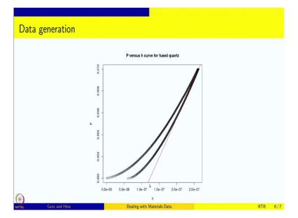
So this is how the load versus depth curve looks. So this is the loading part and then it is held for a while and it is unloaded, this is the peak load and the depth at peak load is this quantity and we are going to fit the unloading part to a straight line and we are going to fit slightly after this max, we come a little bit down and take the data and do the fitting and the intercept actually gives the depth that you get from this slope line.
