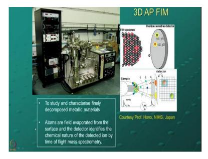
Now, where is the application for all this distribution in material science we say that dealing with material science data. So, here it comes the all answers I would like you to find out but here is case of three dimensional atom probe field ion microscopy. This is the machine and the purpose is that you take any specimen any metallic or any material specimen.
