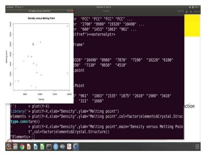
We can give a name to the plot, so we can give a name and as you can see density versus melting point name is given. So you can do all this things and we have also colour coded the points in the scatter plot to show the different crystal structure.
