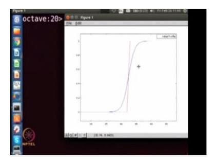
As you can see the initial profile is taken to be this half is one and it forms a nice tan hyperbolic interface in the case of alençon equation also so alençon equation in 2d if you try to solve. The same problem it is not stationary like this will move so in this case also you can show that the solution is tan hyperbolic and in the case of moving solution it is tan hyperbolic of x minus VT that is the velocity of this point if you take into account with time.
