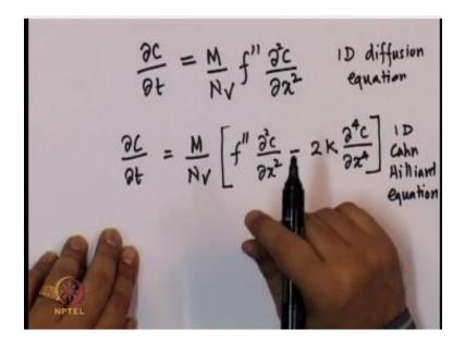
So of course that is written as  $\partial$  by  $\partial$  t is equal to m by NV f double prime del square c by del x square this is one d diffusion equation the difference is that usually this quantity is called diffusivity d but now we are writing the diffusion equation in terms of mobility and the free energy per atom and its curvature and the e n v is the total number of atoms in the given volume so it's typically our garage number.
