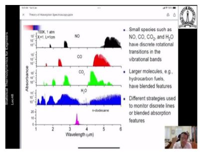
The small species, you can, you see they have discrete rotational transitions in the vibrational bands. Larger molecules have blended features. So, all these are absorbent of NO, CO, CO2, water, and that last one is in total.
