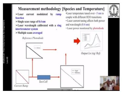
So, this is how this is done. The laser current is modulated by a ramp function. Scan range is typically about 0.4 nanometres. So, very short. The laser wavelength is calibrated usually
