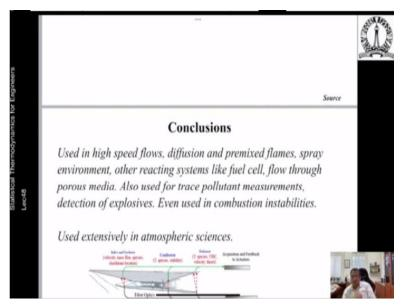
So, used in, this is used in high speed flows, diffusion, premix, flames, spray environment, reacting systems like fuel cell, flow through porous media, also used as trace for pollutant measurements, detection of explosives of the airports. So, even used in combustion instability, it is extensively used in atmospheric sciences. So, all these things are something that that is done through absorptions spectroscopy, which is rather easy.
