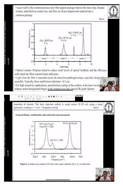
So, you can also have, a complete sensor architecture in which you can have different lasers which are coupled, fused and then so the beam that comes out of it has got combination of all these wavelengths, and then it is passed through your experimental setup, which is shown right over here. And then you detect the signal and then you again, different, you can measure all species at one particular go multiple species at one particular go.
