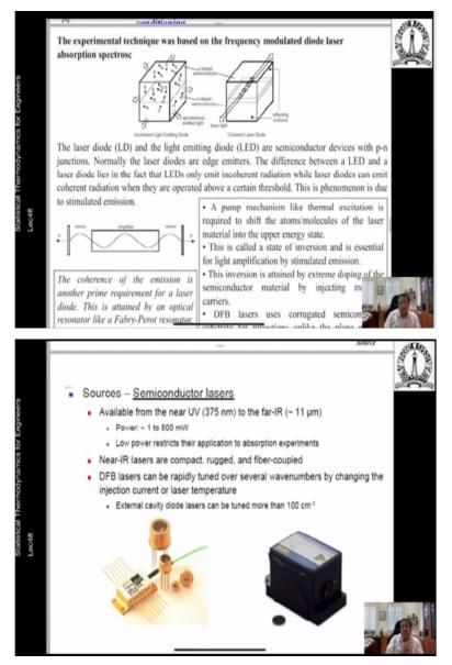
So, it is usually done by a frequency modulated diode laser. So, the diode laser, if you do naught know what a diode laser is, these are semiconductor devices with PM junctions. So, normally the laser diodes are edge emitters. So, difference between an LED and a diode lies in the fact that LEDs only emit incoherent radiation, laser diodes emit coherent radiation when they are operated about the first circuit threshold.
