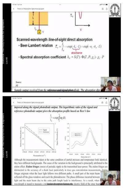
So, this is the line of site-based direct absorption. So, it has to come out, so it is averaged over the distance 1, remember that distance 1 that is over the distance over which we have kind of averaged it out. So, and it is the log algorithmic ratio. So, you can see the two different measurements, for example, they look very identical. The base is sometimes shifted, but that is not a problem. You can just move it up and down. So, that is naught an issue at all.
