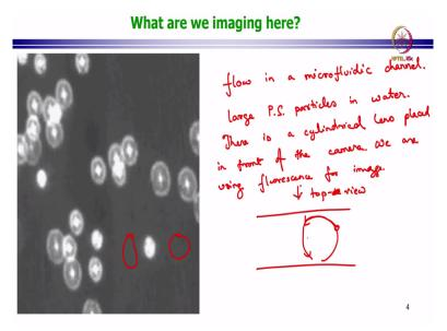
So, now I am going to show you a slightly different type of imaging this is done in an optical microscope, this is flow in a microfluidic channel. The microfluidic device is not visible. These are large polystyrene particles for which I will just write P S the P S meaning polystyrene particles which are neutrally buoyant in the water. There is a cylindrical lens placed in front of the of the camera and we are using fluorescence for imaging.
