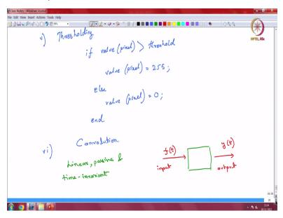
There is a very common operation that people do which is called thresholding. Now the thresholding also you can define a complicated algorithm for that, but usually a simple thresholding operation is you look at the pixel value and you define a certain threshold. And if the value at that pixel at that particular pixel is greater than the threshold then you set the value of pixel to the max.
