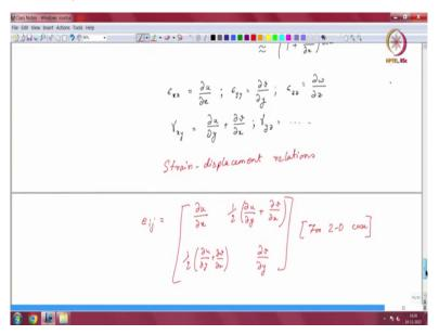
So, now these are also called the strain displacement relationships and in matrix form. When we write this down, we usually would say e ij is in two dimensions if I have to write this it is this matrix. So, we put a half here for 2D case. So, this shows you this the reason I did this geometrical method is simply because this is something that you might have come across in a textbook.
