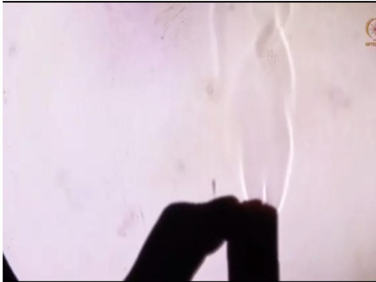
Now, if I partially raise this lighter, then there are combustible gases that are coming out of the lighter that have a different refractive index than the surrounding air. These gases are not visible by naked eye, but this can be easily captured through this Schlieren imaging setup. So let us see how it looks.
