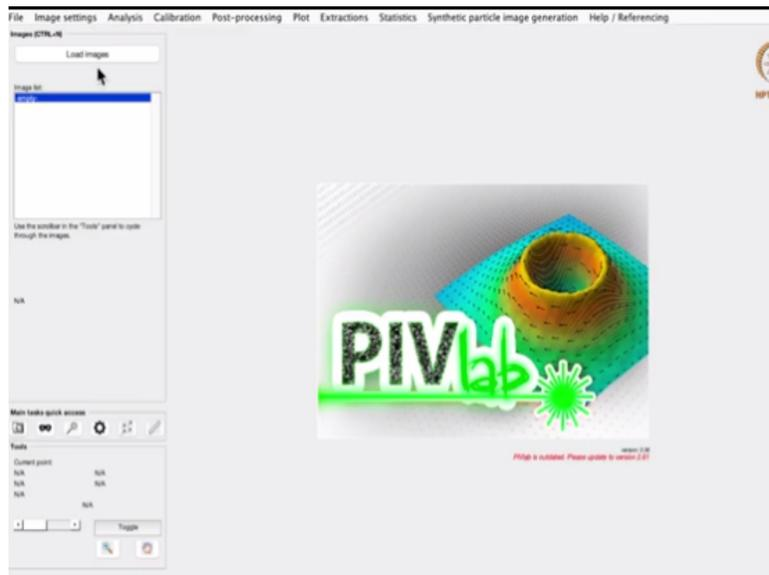
Okay, this is the window for PIV lab application. It is a very interactive software and there are lots of options available, but I am going to walk you through the key steps required to do the PIV analysis. So it majorly consists of three steps. First is pre-processing, then processing and then post-processing. In the pre-processing part, we do the preliminary image processing on the PIV recording, where we get rid of noises to make it suitable for PIV analysis.
