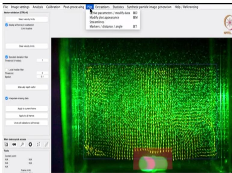
Okay, now it looks better. So you can see the velocity vector field on the plane of illumination. Again, there are some vectors which you can see on the bottom left corner, which are completely different from the nearby vectors and that is how we spot the spurious or the erroneous vector. Now we need to get rid of these vectors and that is our post processing part. So under this post processing menu, we go to the vector validation.
