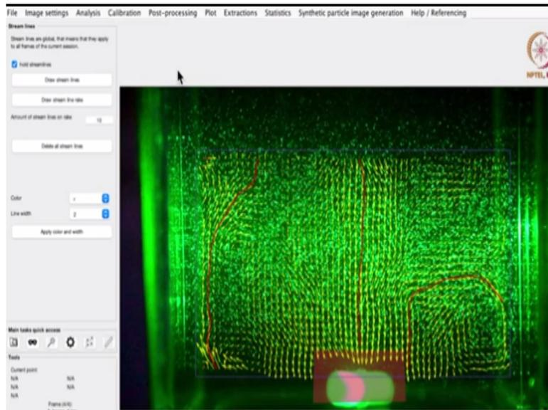
Okay, so now you can see the streamlines passing through the points that I selected earlier. There are similar other interesting option under this derived parameters and post processing and then calibration. Using calibration you can put an image to convert the pixels into some metric unit or any unit of your requirement. So I encourage you to go and try these options on your own.
