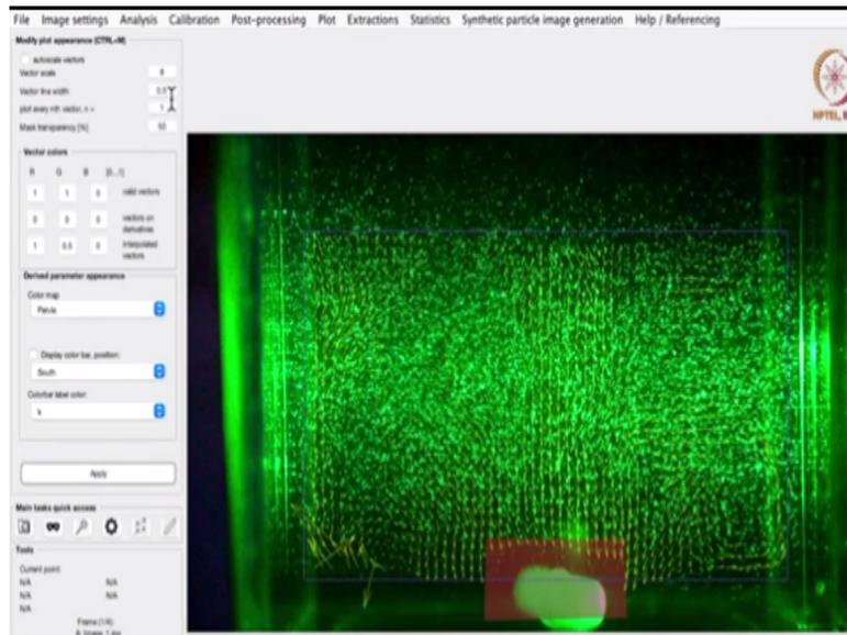
So right now the vector field is plotted in green and the background is also green. That is why they are not properly visible. So what we can do is, we can go to this plot menu, modify plot appearance. So the vectors are plotted in green, let us try to plot it in yellow, then apply. We can also increase the line width of these vectors. Let us make it around 1.
