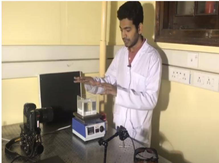
This is our specimen. It is a transparent fluid tank and I have kept water in it. It is kept on a magnetic stirrer and there is a magnetic bead inside the water and when I turn on this stirrer it rotates and it creates a flow field inside, the water that is kept inside this tank. Now I have also kept tracer particles in this water and I have used glass spheres with size 9 -13 micron in diameter as the tracer particles and this tracer particles are ordered from Sigma-Aldrich.
