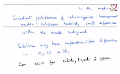
So here I will try to introduce a word called Schlieren, which I will say that the gradient disturbances of inhomogeneous transparent media are called Schlieren. They are relatively small differences, relatively small differences over the background. So we are not talking about very large differences, very small differences over or within the overall background.
