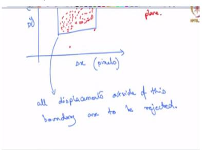
So you draw this, so all displacements outside of this boundary are to be rejected, okay? So this is one way.
