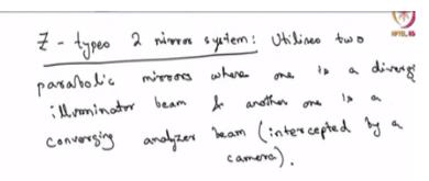
Now you can have different types of Schlieren imaging. One is also called the Z-type two mirror system, which is what we are going to see in one of the lab tours that we will give you. So there are different types of systems possible using lenses or mirrors.
