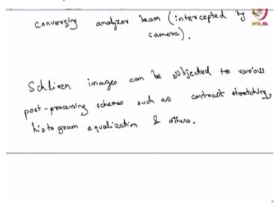
So now Schlieren imaging because they are Schlieren's images can be subjected to various post processing schemes such as contrast stretching, histogram equalization and others, okay? So the only thing you must take care of in the post processing of Schlieren images is that the image should not become distorted.
