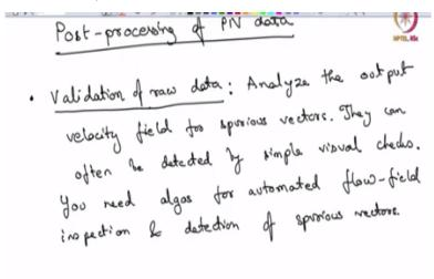
We are going to look into the post processing of PIV data, okay? Now once you do the do the image analysis and you get a velocity field, you must do validation of raw data. So you will get an output from your software and but you must check it right, so that is what validation means, validation of raw data, which means that analyze the output velocity field for spurious vectors..
