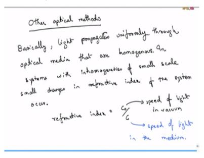
But I just wanted to have a small discussion about other optical methods. Now basically techniques such as shadowgraphy and Schlieren, what they do is they use the idea that light propagates uniformly. So light propagates uniformly through optical media that are homogenous, sorry that are homogeneous. But when light encounters inhomogeneities then the speed of light changes in some sense in relatively in these cases.
