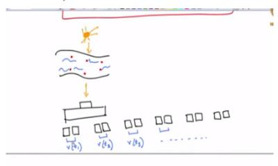
You have let us say, some system in which there is a flow that is happening. And there are some tracking particles, seed particles, there is a source of light somewhere. And this light is eliminating our fluid. And then finally, this is being captured by some camera. And hopefully, it is a special type of camera where it is clicking an image pair. And then after some time, another image pair, after some time another image pair.
