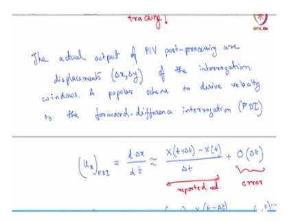
And finally, when you have the actual output, you do get displacements delta x and delta y. And now you have to use numerical schemes in order to get a velocity field, which is a derivative of the displacement field and the time derivative of the displacement field to finally get the velocity map.
