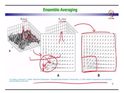
So for example, this is the result of this velocity field is gotten from the correlation, the correlation calculation on the left, whereas here this image this velocity diagram is a result of the ensemble averaged correlation. So you can see here there are a lot of vectors which are spurious vectors right. So you have this flow, but then you suddenly have a vector that is pointing in the opposite direction.
