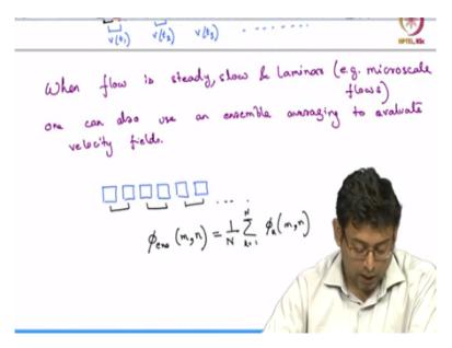
Now one special case I want to discuss is what happens when flow is steady, slow and laminar, example microscale flows. One can also use an ensemble averaging to evaluate velocity fields. What do I mean by that? Well, so in such a case, you can use a normal camera and then you can take images such that the images are equally spaced away from each other.
