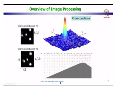
And we discussed about the idea of cross-correlation between different windows and how for example, we can use these sub sections of images and produce and calculate cross-correlation to find out the displacement of particles from one frame to another and how this cross-correlation peak tells us how much displacement has occurred between two images.
