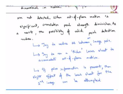
So if you have a situation where you have significant out-of-plane motion of the tracer particles or the basically the flow is three dimensional, strongly three dimensional in nature, what you can try to do is, one of the first things you can try to do is try to reduce the delta t between image pairs. And deliberately between an image pair, okay? So this is the delta t between two successive frames
