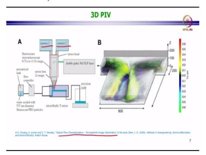
So with that I just wanted to also let you know that there are different techniques which do use three directional particle image velocimetry. One such method is the use of confocal imaging, where you can image different planes successively, and make sure that every plane has a very small depth of field and then you go on tracing different z planes with your microscope.
