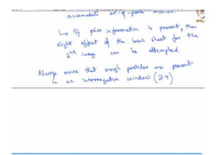
And always you have to ensure that enough particles are present in an interrogation window, in an interrogation. And enough particles usually means that greater than 4 equal to or rule of thumb 4, 5 the more the better. But it should not go below 4 or 5. Then it does become a problem.
