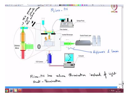
So, this is for micro particle image velocimetry you have let us say a laser here that is now going to come through a diffuser. So, there will be a diffuser element here and some lenses diffusers and lenses. I will explain what they are for and when they come in and go through your lens into and illuminate your sample. Now this light if I were to use the green light line here this green is going to illuminate this entire volume over here.
