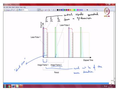
Briefly what a synchronizer does is it ensures that the images and the laser pulses and the imaging is synchronized and usually what happens in a synchronizer is that a control signals are generated. So, this is a diagram which shows what schematically what happens. So, for example, if you have a synchronizer what it will do is in this particular schematic you have three control signals that are being generated by the synchronizer.
