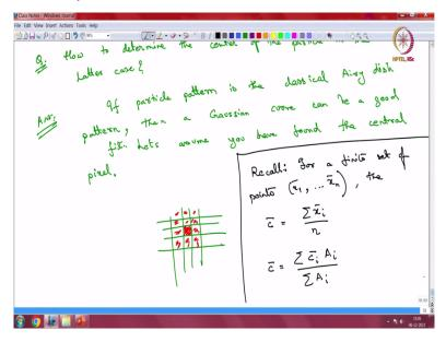
So, the question we are trying to ask is how to determine the center of the particle in the latter
