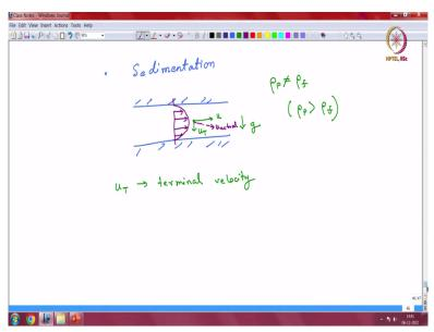
So, another problem that surfaces quite often is the problem of sedimentation. Now again I will take a particle in a channel. Let us say this time there is a parabolic flow through this channel. So, this is the underlying flow field and some particle now has to follow this. So, you have a particle you have a tracer particle that now has to follow so it is getting entered in this direction so it will have some velocity along your positive x direction.
