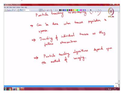
This is also known as particle tracking velocimetry. Now the reason I want to introduce PTV is also when I introduce PIV I am going to make a very strong distinction between PTV and PIV. So, this can be done when tracer population is sparse and we will we will see what sparse means when we encounter PIV we will see that the population there is no longer sparse.
