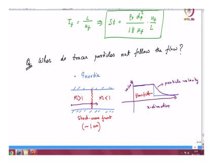
So, the question we are asking is when do tracer particles not follow the flow? By the flow I already mean the underlying flow field so that is sort of understood I do not have to elaborate upon it. So, intuitively the first would be the particle inertia. So, if the particle had no inertia at all associated with itself it would always follow the flow field irrespective of how sudden or how difficult the flow field is to follow.
