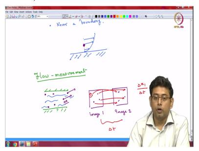
So, we are now going to get into flow measurement so we understand that we are going to measure flow by the use of proxies which are tracer particles and these proxies are going to help us visualize the underlying flow field. Now one of the most obvious ways of measuring a flow is to let us say you have a condition like this where you have some fluid and then you have these particles that are there.
