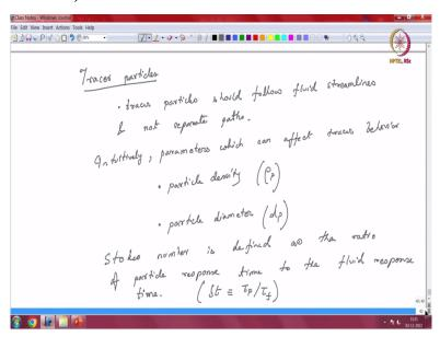
So, what I need a tracer particles and assumption is going to be that tracer particles should follow fluid stream lines or fluid particles as they move and not separate paths and not some of its own path. So, intuitively what are the things that can affect this? So, intuitively the parameters which can affect tracer behavior would be particle density. So, my row of the particle of the tracer so I will just put a p here.
