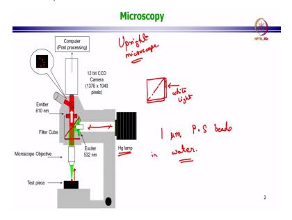
Here I have drawn an upright microscope. Now the upright and the inverted microscopes are different only in the way the lenses and the optical system is placed with respect to the to the object, but the operating principles are more or less the same. So, that is why for completeness I wanted to show you how an upright microscope looks like and what I am going to show you here is the principle of setting up the optical pathway for let us say a fluorescent imaging.
