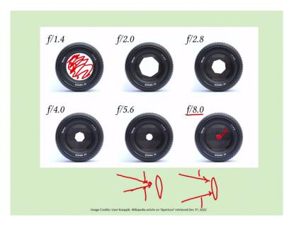
So, in the lab session one of the things Naveen is going to show you is the effect of aperture and this image which is not mine and I have given the image credits at the bottom here. The effect of different f numbers is shown so as you can see this is f 1.4 and this is f 8.0 and it is sort of obvious what is happening. This is the area through which light can pass at f 1.4 and corresponding here this is the area over which light can pass at an f number of 8.
