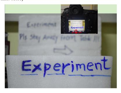
This is the first image and we can see that the f number here is f 5.3. So, when you input the number of 5.3 this is again a number that you can control from the camera body, the lens is such that it is motorized. So, the coupling is such that the moment you input this number the camera forces the lens to operate at f 5.3 and this is the image that you get. This is the object that was placed in front.
