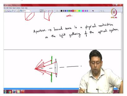
Another topic to quickly discuss before we step into the lab is the idea of an aperture. Now an aperture in a very broad sense is a physical restriction on the light gathering capacity of the optical system. So, how would you want to make one. So, for example, if you have a lens let us say and you have an object here that is sending out light rays in every possible direction then in the regular case this light would be intercepted by this lens.
