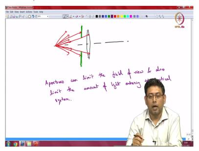
So, apertures can limit the field of view and also limit the amount of light that is coming to the system; so the amount of light entering the optical system. So, if I make my aperture smaller and smaller, for example, in this particular case I can make it smaller and smaller the image becomes dimmer and dimmer because less and less light is processed by my imaging system.
