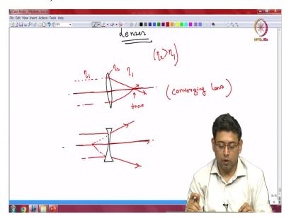
Now the thin lens is a simple version of what type of lenses we encounter today and the reason they are important is because in thin lenses the image that is formed by the optical system that can be understood simply. So, there are two wide widely used type of lenses one is something called as the convex lens and the other is the concave lens. So, this is for example the top image that I am showing you here.
