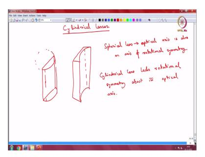
There is a one important type of lenses that you will also encounter called cylindrical lenses. Now in cylindrical lenses as the name suggests the lens is actually part of a cylinder. So, for example, this could be a cylindrical lens. So, this for example is a is a cylindrical lens. So, you can see that this if I had extended this further this would have been a sort of a cylinder right here.
