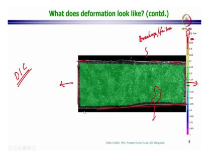
Here the deformation is going to be small enough for you to see for a small enough for you to not be able to see. This is video that I am going to play this exemplifies a an experimental technique called DIC which is digital image correlation. I will quickly, explain what you are going to see here. We have again a bar that you in the background, this bar is being pulled again in the two directions and it is undergoing a tensile test.
