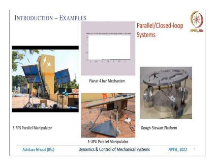
Let us continue with some examples of a parallel or closed loop system. So, this example here which I am going to show you this is a very well-known 3 RPS parallel manipulator. Just to give a little bit of a background, this parallel manipulator is used to track the sun. So, there is a way to collect solar energy and harness solar energy in which basically you put a mirror in and the mirror is rotated or moved in such a way that the incident beam from the sun is focused onto a receiver.
