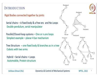
So, let us look at a system of rigid bodies connected together by joints. So, a kind of system of rigid bodies these are sometimes called a serial chain. In these serial chains we have one fixed body and a free end and there are no loops, I will show you what is the loop very soon. A simple example or a well-known example of a serial chain is a double pendulum or even a serial manipulator or a serial robot.
