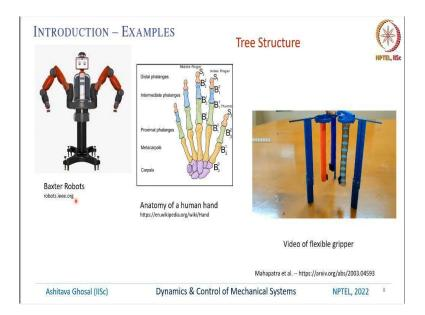
So, a tree structure as I said consists of one fixed body and then there are these arms. So, this is a well-known robot which is called as a Baxter robot this is basically used in many factories. So, there are two arms so just like a human being this robot has two arms and it can manipulate an object it can coordinate and it can pick up objects heavy object with both the arms and so on. This is another example of a tree structure our hands, with these five fingers.
