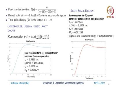
To again meet the same dominant, closed loop requirements. In that case again, we had the same system, the same desired poles, the same third pole at s = -10 and we did a controller design using root locus and a compensator. Please go back and see that the compensator which we designed was 31.4 (s + 4)/(s + 15) and (s + 5)/(s + 18.15). These were designed such that the angle and the angle at that desired poles the angle was -180 degrees.
