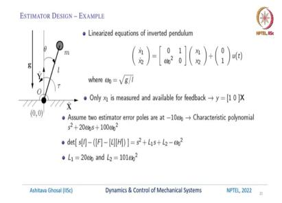
So, after all this theory and general expressions just let us look at a simple example. So, we have this inverted pendulum. The linearized equation of an inverted pendulum can be written in this form. So  $\dot{X_1}$ ,  $\dot{X_2}$  so,  $X_1$  is  $\theta$ ,  $X_2$  is  $\dot{\theta}$ . So,  $\dot{X_1}$  is  $x_2$  and then  $\dot{X}$  is  $\omega_0^2 X_1 + u(t)$ , u(t) is like this torque and this  $\omega_0$  is  $\ddot{Og}/l$ .
