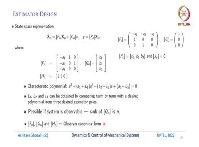
So, the state space representation using the observer, the new block diagram can be written in this form. This  $\dot{X}$ , and I am putting *o* for the observer canonical form, is  $[F_o] \mathbf{X}_o + [G_o] u$
