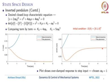
So, continuing so, the desired closed loop characteristic polynomial is  $(s + 2 \omega_0)^2$  and we can expand this as  $s^2 + 4 \omega_0 s + 4 \omega_0^2 = 0$ . The determinant of the closed loop system or the characteristic polynomial of the closed loop system is det (s [I] - ([F] - [G][K])) and remember what is [F]? [F] is  $[0 1; \omega_0^2 0]$  and [K] is  $[K_1, K_2]$  and [G] is [0 1].
