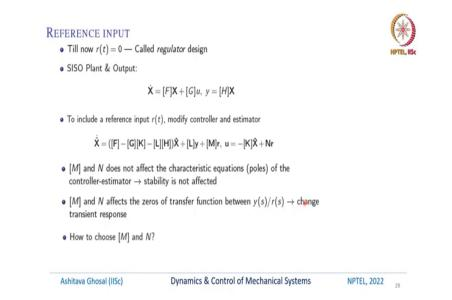
Till now, we have not considered the reference input till now, r(t) was 0. This in control theory is called a regulator problem, so, we have designed a regulator with r(t) = 0. So, for a single input, single output plant and output we have  $\dot{X} = [F]\mathbf{X} + [G]u$ , we have seen this many times now and  $y = [H]\mathbf{X}$ . To include a reference input or r(t) we need to modify the controller and the estimator.
