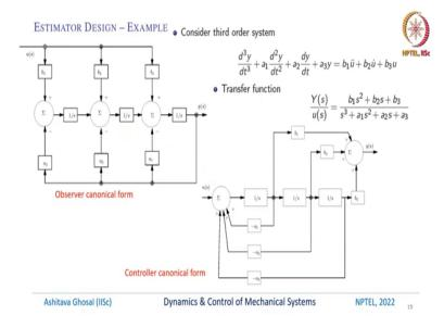
So, just let us look at the estimator design example. So, let us go back and consider the third order system that we had which is  $d^3 y/dt^3 + a_1 y + a_2 y + a_3 y = b_1 u + b_2 u + b_3 u$ . And we had obtained this transfer function Y(s)/u(s) is  $b_1 s^2 + b_2 s + b_3$  and denominator is  $s^3 + a_1 s^2 + a_2 s + a_3$ . So, in the controller canonical form, if you go back and see your notes or previous slides, the block diagram look like this.
