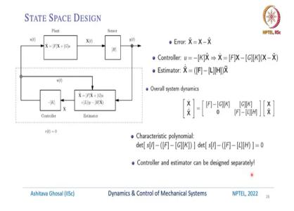
Continuing with the state space design, let us look at the block diagram, so, we have a plant which is given by  $\dot{X} = [F]\mathbf{X} + [G] u$ . There is an input u(t) the output is  $\mathbf{X}(t)$ . There is a sensor, so, we get  $y = [H] \mathbf{X}$ . Then this y is fed back into this estimator because we are only using some
