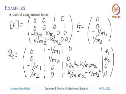
So, we can rewrite in the state space form. We have  $\dot{X} = [F]X + [G]u$ , [F] will be this matrix 4 x 4 matrix, so, we will have  $(0\ 0\ 1\ 0, 0\ 0\ 0\ 1)$ . This element is  $-K/m_1$ , second element is  $+K/m_1$ . This is  $K/m_2$  and this is  $-K/m_2$ . The [G] vector will be  $0\ 0\ -1\ /m_1$  and then  $+1\ /m_2$ .
