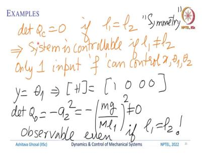
So, hence determinant of  $[Q_c] = 0$ , if  $l_1 = l_2$ . So, this is what I mean by saying that there is too much symmetry -- we have a mass which is going translating and that there are these two pendulums with equal masses but the lengths are also equal. So, it is in some sense, very special and very symmetrical. So, this system is not controllable if  $l_1 = l_2$  and is controllable if  $l_1 \neq l_2$  -- then you could see that the determinant of  $[Q_c]$  is not equal to 0.
