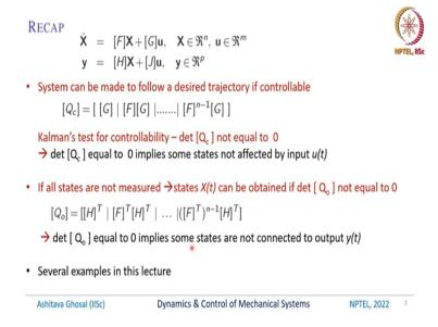
To recap in the last lecture, we had looked at a state space representation of a linear time invariant system given by the state equations which is  $\dot{X} = [F]X + [G]u$ , X is an element of  $R^n$ , u is an element of possibly  $R^m$  and output equation y = [H]X + [J]u, where y could be a  $p \times 1$  vector. Most of the examples we looked at where u was single input and the output y was also one output - so, it was single input, single output systems.
