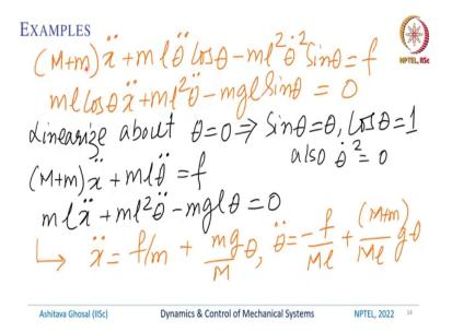
So, the equation of motion looks like this. It is  $(M + m)\ddot{x} + m l \ddot{\theta} \cos \theta - m l^2 \dot{\theta}^2 \sin \theta = f$  and then  $m l \cos \theta \ddot{x} + m l^2 \ddot{\theta} - m g l \sin \theta = 0$ . These are two non-linear equations -- you can see that there is a  $\dot{\theta}^2$  term, there is a  $\sin \theta$  - so, it is a nonlinear- and  $l \sin \theta$  is also there.
