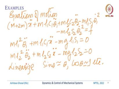
The equations of motion will be three of them because there is one cart and then there are these two pendulums. So, if you do some simple calculations of finding all the partial derivatives and all the time derivatives and then we organize it together, which I am not going to do because by now you should be able to do it very easily, you will get three such equations of motion.
