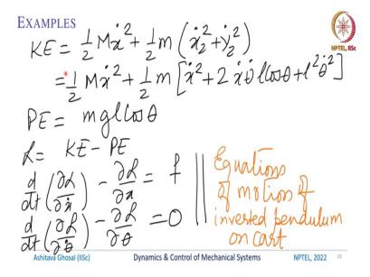
We can find the kinetic energy which is (1/2)M - M is the mass of the cart and small m is the mass of the pendulum bob -- so,  $(1/2) \dot{M} \dot{x}^2 + (1/2) m (\dot{x_2}^2 + \dot{y_2}^2)$ , and you can expand this and we will get  $(1/2) \dot{M} \dot{x}^2 + (1/2) m (\dot{x}^2 + 2 \dot{x} \dot{\theta} l \cos \theta + l^2 \dot{\theta}^2)$ . This is very, very straight forward.
