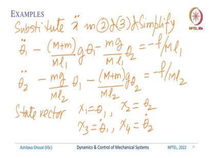
So, we can substitute  $\ddot{x}$  back into (2) and (3) and simplify. Basically, what have we done? We have gotten rid of  $\ddot{x}$  -- from those three equations in three unknowns, we have two equations in two unknowns. The first equation is
