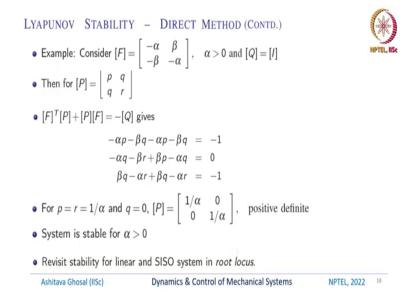
Example so, let us take a simple example of F which is a 2 by 2 matrix it is  $-\alpha \beta$ ,  $-\beta - \alpha$  and  $\alpha > 0$ . So, we choose [Q] as [I] and the elements of *p* are *p q*, *q r* it is a symmetric matrix. So, if you solve  $[F]^{T}[P] + [P] = -[Q]$ , you will get these three equations in  $\alpha \beta p q$  and *r*. So, you will get  $-\alpha p - \beta q - \alpha p - \beta q$  as -1 and so on.
