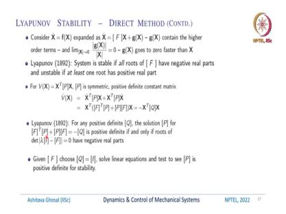
So, the Lyapunov stability theorem of finding a V(X) which is positive definite and V(X) which is negative definite is sort of not so easy to apply. Because we have to keep on trying for different V(X). So, Lyapunov in 1892 went on further, he proposed the following or he showed the following. So, let us consider a non-linear system which is given by  $\dot{X}(t) = [F]X$ .
