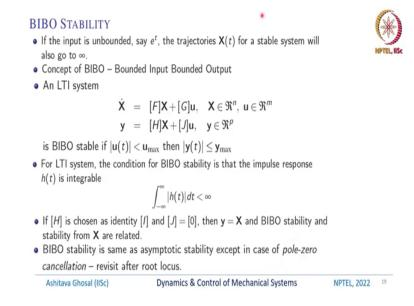
So, till now we looked at stability according to Lyapunov. So, there are other ways or other definitions of stability, one such definition is called BIBO stability. So, BIBO stands for bounded input bounded output and the basic idea is the following. If the input is unbounded say  $e^t$ ,  $e^t$  the function goes to infinity as t tends to infinity. And if the input is unbounded, the trajectory X(t) for the stable system will also go to infinity.
