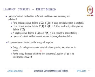
So, let us continue with this Lyapunov stability. So, Lyapnov's direct method is a sufficient condition not necessary and sufficient. Remember in many theorems in math so, for example, if you want to find the maxim optimization if you are interested in optimization we say a function is maximum when the first derivative is 0 and it is sufficient condition is when the second derivative is < 0.
