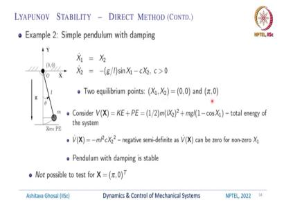
So, let us continue with the simple pendulum with damping. So, for this pendulum with the mass *m* and length *l* and gravity acting this way, I can write the state equations as  $\dot{X}_1 = X_2$ ,  $\dot{X}_2$
