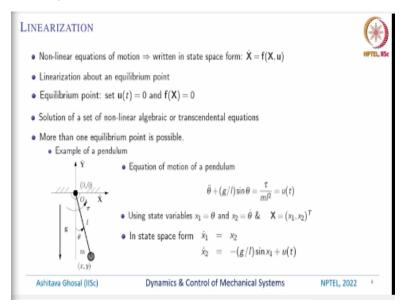
So, let us look at an example of linearization. So, we have this simple example of a pendulum, so we have this rod a mass less rod with the mass at the end and it is rotating about this z-axis, so the rotation angle is  $\theta$  from the vertical. There is also gravity which is acting here and we will also assume that there is a torque which is acting at this joint. So, there is a motor which is applying this torque.
