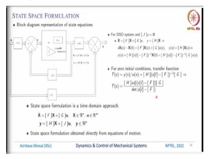
So, in general if you have a system which is X = [F]X and then you have y = [H]X + [J]u, so you have  $\dot{X} = [F]X + [G]u$  and y = [H]X + [J]u. We can also write it symbolically in a block diagram form. So, this is the block diagram representation of the state equations. So, what do we have? We have u which is coming in, so this is [G]u and then we also need to add [F]X, so we will get  $\dot{X} = [F]X + [G]u$ .
