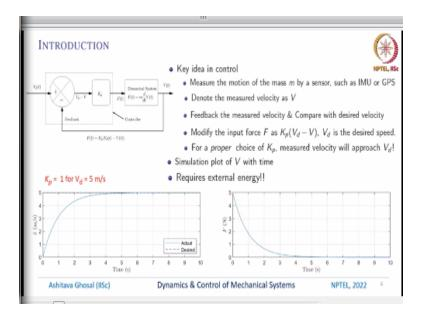
So, the key idea is the following, we have a dynamical system which is given by  $F(t) = m \frac{dV(t)}{dt}$ . So, the input to this dynamical system is this force which could be a function of time and the output is the velocity. So, what we are going to do is that we will measure this velocity of this mass and feed it back. So, what do we mean by feed it back? We will have some desired velocity; remember we want the velocity to be constant.
