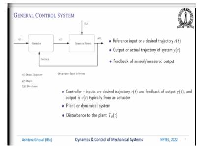
So, the general control system looks like this. So, we have a controller then we have a desired trajectory which is r(t). In the previous example the desired trajectory was 5 m/s. Then the output of the controller is u(t), this is sometimes also called as the actuator input to the system. So, we have to apply some force or later on we will see we have to apply some voltage to this dynamical system.
