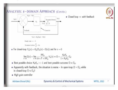
So, if you have closed loop with feedback then what do we have that this voltage which you are applying to this plant is  $K_p(\Omega_d - \Omega)$ . So, again in steady state we are going to assume that as  $s \rightarrow 0$ , the plant is  $\frac{K}{F}$  which is  $K_0$ . So, now for closed loop this voltage is  $K_p(\Omega_d - \Omega)$ . So, we can see it is written here Voltage applied is which is this is  $K_p$  into whatever is coming into the block which is  $\Omega_d - \Omega$ .
