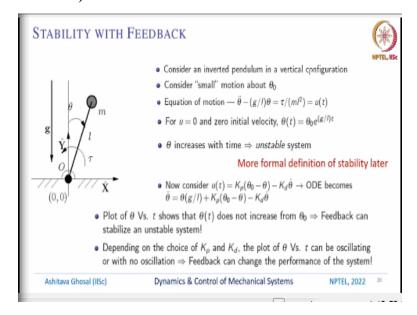
Let us continue, as I said one more purpose of controller is to stabilize an unstable system. So, again we will do these things in much more detail and rigorously later on but right now I am taking a very simple example. So, this is what is called as an inverted pendulum, so I have a joint here, a rotary joint and then there is a rod and there is a mass and gravity is acting downwards.
