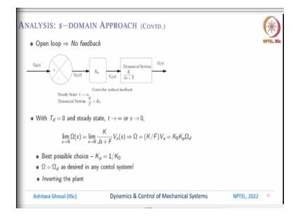
So, let us see what happens when you have open loop and no feedback? So, when you have open loop and no feedback you have  $\Omega_d$  which is coming in, there is no feedback, so the output of the summation block is still  $\Omega_d$ , this is  $K_p$  and there is output of this controller is Voltage and we get this. So, again with  $T_d = 0$  and in steady state which means  $t \rightarrow \infty$  or  $s \rightarrow 0$ , so what is  $\Omega(s)$ ?
