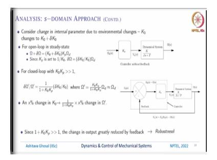
So, let us continue, let us see what we can achieve by doing this feedback. So, first thing is let us consider the open loop system and remember we have chosen  $K_p$  as  $1/K_0$ . So, in the open loop system controller without feedback, I have a desired  $\Omega_d$  desired speed this  $K_p$  is  $1/K_0$  and then the output is the voltage which I am sending to the dynamical system and we have the speed which is the output of the link.
