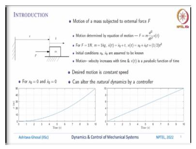
So, let us look at an example, this is an example of very simple example of a mass m in which there is an external force F which is acting from left to right. The mass is at a distance x from some reference and it has an acceleration  $\ddot{x}$ . So, the motion of this mass subjected to an external force is given by this equation of motion which is F = m a, everybody knows this, it is very simple straightforward, so this is  $m \frac{d^2 X}{dt^2}$ .
