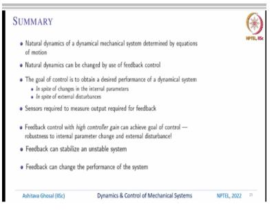
So, in summary the natural dynamics of a dynamical system is determined by the equations of motion, f = ma. So, if I tell you what is f, I can at least conceptually find out what is a and then I can integrate a to find velocity and I can integrate again to find the position, I can plot position as a function of time, so same thing if it is rotating. If you have  $\tau = I \alpha + \omega \times I \omega if I$  give you the torque I can.
