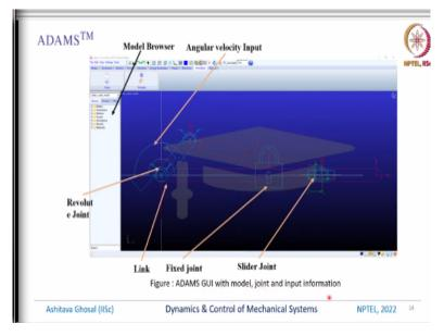
So, this is a student version, so there is some ghost pictures at the back but basically what we have done is we have created a revolute joint which is this then there is a crank, then there is another rod, connecting rod and then there is a slider joint. So, this is one link which is connected to the fixed ground then there is a slider joint and the top of the slider joint is connected to this place with another link and we are going to give a angular velocity input.
