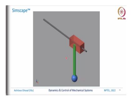
So, here is the model of the cart with the pendulum. (Video Starts: 47:22) And then you can see that while it is moving this way and that way, this pendulum will also oscillate. So, this is a very short simulation how do you know that this is correct that this is reasonable? The answer is people have worked on it for a long time they have tested, maybe they have even verified with experiments.
