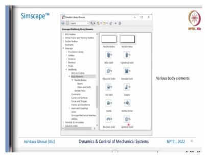
So, we choose this various body elements we can have a solid, we can have a cylindrical solid and various shapes are possible. And then we can have sensor, inertia, revolved solid, spherical solid various possibilities are there, so we can pick the various body elements.
