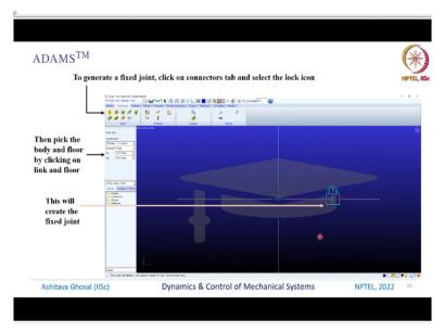
You also need to say which link is fixed. So, in your slider crank mechanism the base link is fixed. So, to generate a fixed joint click on the connectors tab and select the lock icon then pick the body and the floor by clicking on the link and floor. So, then this body and the floor
