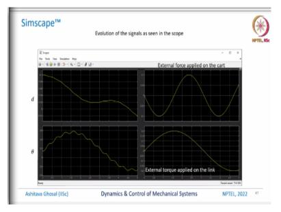
We can also plot the thetas and the d. So, this is the plot of theta as a function of time, this is a plot of d as a function of time, this is the plot of the external force, remember there was a
