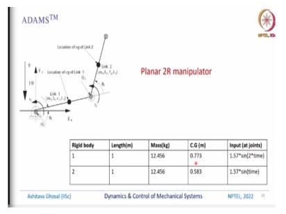
So, let us take another example which is this planar 2R manipulator and for this planar 2R manipulator we are choosing mass and length similar to what we did for the simulations using MATLAB and the CG is also similar. The input however is different, in this case the input at the joint is 1.57 into  $\sin \sin (2 * time)$ , so it is  $\sin \sin 2t$  and this is 1.57 into  $\sin \sin t$ , so this is like  $\pi/2$ .
