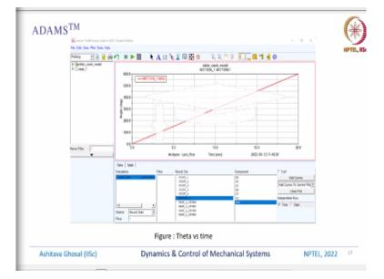
We can also find out the plots of various components after the simulation. So, what you can see is that the angle is going from 0 to 600 because we are rotating at 30. So, in 20 seconds it went from 0 to 600, so it is 30 degrees per second, that is what was the input. And we can see all these things by going to this block here which tells you that this is motion, this is angle and you can add curves to plot here.
