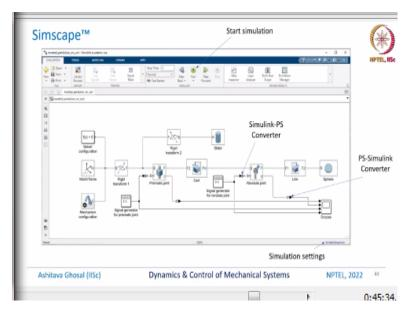
So, once you do all this then you can make a model and in the model you have some kind of a solver configuration. We have this reference coordinate system, then we have this mechanism configuration and this is rigid transform then you can give an input. For the input for the prismatic joint is some oscillation, then we have the cart. So, this kind of block diagram is very, very similar to what we do in Simulink or what we do in control system analysis and design using Simulink.
