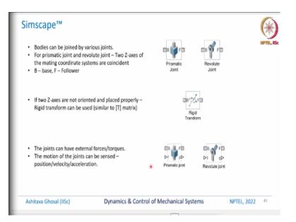
So, we pick bodies and they can be joined by various joints. For prismatic joint and revolute joints 2 Z-axes of the mating coordinate systems are coincident. So, we have one rigid body here and we have another rigid body inside and the Z axis of both these 2 rigid bodies are coincident. Same thing with the revolute joint and this is we have discussed earlier most of the time the Z-axis is the joint axis and that is what it means here.
