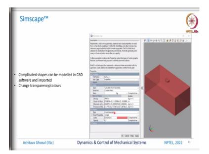
We can also make complicated shapes in a CAD system and import them. So, for example we can have a block with some small protrusion here. And again once you tell them that these are the dimensions this is the density it will find center of mass and various other things, inertia is also there.
