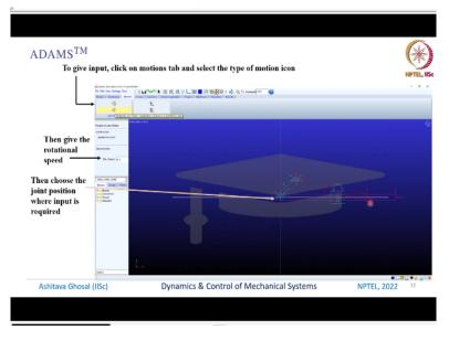
So, once you have this input link which is this and then you have another link and then this third link is the fixed then we need to give input, to give input we click on the motion tab and select the type of motion icon you want. So, if you want to give rotational speed then you can give the speed in this case we have chosen as 30. Then you choose the joint position where the input is required.
