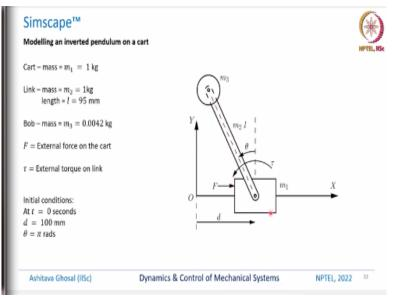
So, in Simscape we will take this example of a modeling of an inverted pendulum on a cart. So, this is a very classical problem in multi-body dynamics and control. So, basically what you have is a cart, so it is like a cart with wheels, it can go along the X direction and then on top of that there is a pendulum. So, the mass of the cart is 1 kg, the link length is 95 millimeters which is chosen the link mass is 1 kg and the mass of the bob is very small, it has been chosen arbitrarily.
