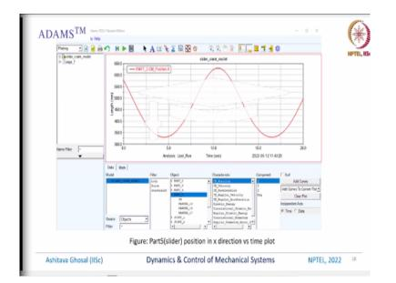
We can also plot the location of the slider; this slider is going back and forth. So, that is part number 5, it tells you that we have this slider crank model and this part number 5 is the slider part number 1 is something else, part number 2 is something else, I want to see the motion of this slider and we can see the position, you can also see what is the velocity, acceleration, kinetic energy various things.
