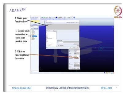
So, once you do all this you can double click on the motion icon here to open a joint motion pane. So, here what you can do is you can click on the function and give your own function. So, I want 1.57 into sin sin 2t for the first joint, how do I do that? You open this and there is
