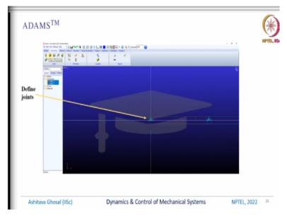
Then we need to put the joints. So, we define one rotary joint which is at the origin and another rotary joint which is a distance of 1 meter away because the lengths are 1 meter. So, we will pick rotary joints and put it here, very similar to what we did for the slider crank mechanism.
