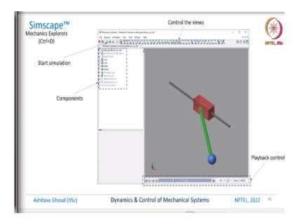
So, once we have connected all these things we can do simulation and inside the simulation you have various components. You can see that we have a cart which is actually this in this case then we have this link, then we have this slider that is between this and this there is a sliding joint and this is a sphere. And then we can see all these various control the views how we can move and then you can simulate.
