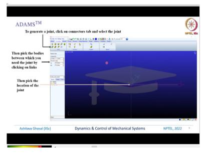
So, let us see how we can generate this slider crank mechanism. So, to generate a link we click on the bodies tab and select a link. So, we can select this link then define the dimensions of the link. So, you can see that this is of this length, width and depth. So, you can type in numbers. So, this is 15 centimeters and some 4 centimeters and some 2 centimeters.
