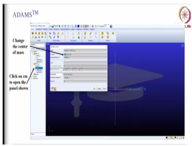
So, we can also change the center of mass and again we can click on this and open a module and there you can say that this is model 1 and these are the center of mass and you can type it and change the center of mass. So, this is now the link 2R robot, so if there are 2 of these and we can change the center of mass, the mass of each link and so on.
