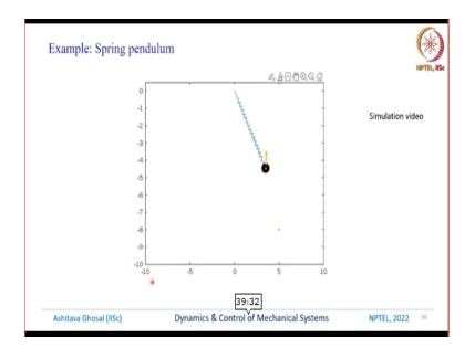
(Video Starts: 39:34) So, here is a video of this spring pendulum and you can see this animation of this mass which is the bob as it is going around. So, what you can see is the spring is lengthening and shortening, so unlike a pendulum there is a spring which is here and the spring can go in and out and this mass can also go in and out. So, this is the simulation which is obtained after solving those 2 differential equations. (Video Ends: 40:07)
