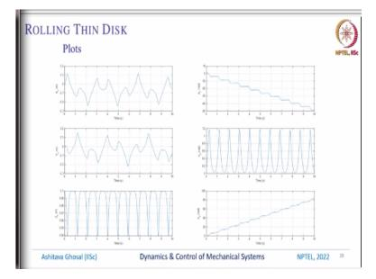
We can also now plot the center of the disk, how it is moving? The Y coordinate, the X coordinate, so this is the X coordinate, this is the Y coordinate and this is the Z coordinate. And this is the way the Z coordinate is changing with time, the simulation is for 10 seconds, so the Z is sort of approximately understandable it has come to 0 go back up and down, it keeps on doing this.
