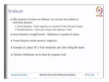
So, in summary after the equations of motion of a multi-body system are obtained one can solve 2 problems in multi-body dynamics. One is this is called as the inverse dynamics problem which is that given trajectory as a function of time, find joint torques. This is just simple substitution on the right hand side of the equations of motion. And the next one is forward dynamics which is given the joint torques, find the trajectory in time.
