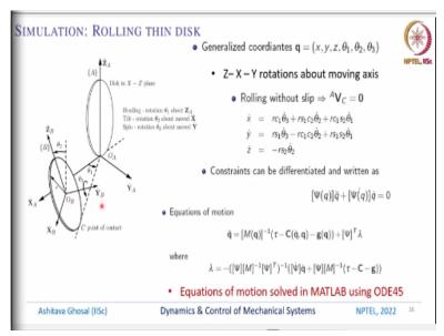
Let us continue, let us look at this simulation of the rolling disk. So, the first simulation was 2R robot with no constraints, the second simulation of the 4-bar mechanism had these loop closure
