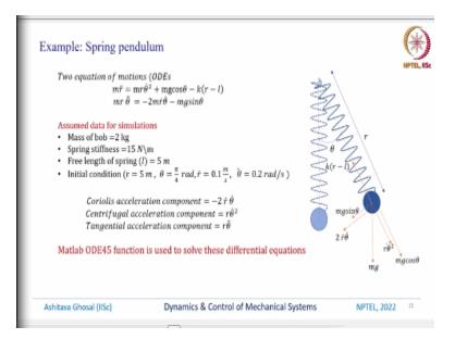
Let us take some examples now. So, another example is that we have worked on earlier which is called the spring pendulum. So, basically we had a mass here which is mounted on a spring, the free length is l and then once the spring is compressed we have a force which is k(r - l). And there is gravity acting and then there is these components  $mg \sin \theta$ ,  $mg \cos \theta$  and also we have this centripetal term and we have this Coriolis term.
