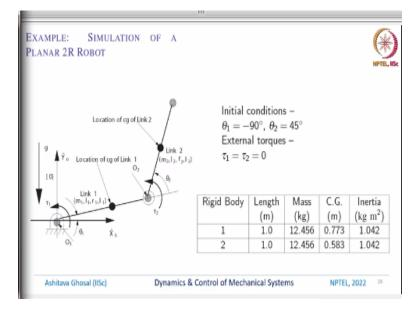
So, once we have those 4 first order equations in the required state space form we can give some initial conditions. So, for this simulation we are choosing  $\theta_1$  as -90 and  $\theta_2$  is 45 degrees, so what does it mean? This link is hanging down because it is -90, so this angle is -90 and then  $\theta_2$  is 45 degrees, so we have a link which is hanging down and the second link is like this at an angle of 45 degrees and there is no torque.
