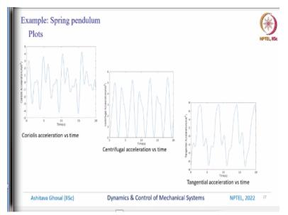
And as I said I want to plot the various acceleration, just to get a feel for what kind of numbers we are talking about. So, the coriolis acceleration from 0 to 20 which is the motion of this bob
