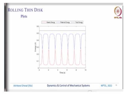
And we can again check that the sum of the kinetic energy and the potential energy is constant. So, again the kinetic energy is shown here, this is the potential energy and the sum is this and you can play around with these codes. So, the TA will put up this code in some available place, you can try it with some different initial conditions and you can see what the disk is doing.
