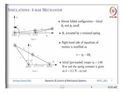
We can also simulate the 4-bar mechanism. So, we have derived the equations of the 4-bar mechanism. And what I am going to do is we are going to place the 4-bar mechanism in this almost folded configuration. So, the first fixed link is this, the second link is this way, the third link is this way and the fourth link is this, so this is exaggerated a little bit. But basically all the 4 links are lying along the *X* axis this is called as the folded configuration.
