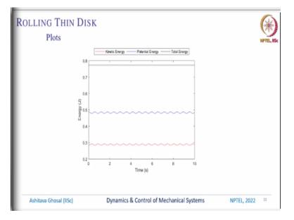
And again to check whether this simulation is correct or not, we can plot the kinetic energy which is this red which is oscillating like this, the potential energy which is oscillating like this. So, remember the disk is not tilting too much; it was tilting a little bit, so hence the potential
