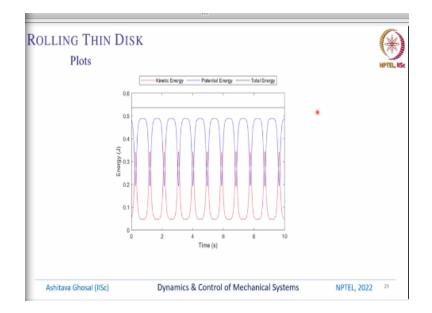
How do we know all these simulations are correct? One test is that we need to ensure that the total energy of the system is constant. Remember, there is no external forces, so whatever is the initial starting energy which is the kinetic energy and the potential energy, we know what is the potential energy it is like  $mg r \cos \theta_2$ , we know what is the kinetic energy, there is an expression for the kinetic energy which I have shown earlier.
