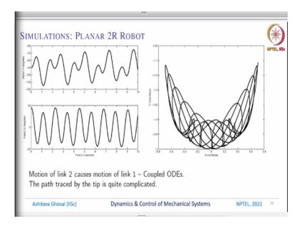
We can also plot actually  $\theta_1$  and  $\theta_2$  as a function of time. So, what you can see is  $\theta_1$  is doing all kinds of things like this, so it is not a simple harmonic motion although we do not should not expect a simple harmonic motion like a sine wave. The second link is little bit more periodic because again it is not because what you can see is the amplitude is changing as we go along. The first link is definitely doing interesting things. So, why does this happen?
