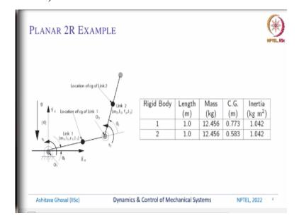
So, let us take an example and again we will use our simple example which is the planar 2 degree of freedom of 2 rigid bodies connected by 2 rotary joints. So, there is a link 1 and a link 2 and again the link 1 is specified by mass, length, location of CG and inertia, likewise link 2 is specified by mass  $m_2$ ,  $l_2$ ,  $r_2$  and  $I_2$ , again  $I_2$  is the z component of the inertia which is of relevance here because this is a planar motion.
