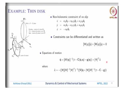
And then we can continue and derive the equations of motion and then we can take into account these non-holonomic constraints of no slip. We can differentiate these constraints standard approach, we get  $[\psi]\ddot{q} + [\dot{\psi}]\ddot{q} = 0$ . So, this is like  $\psi \dot{q} = 0$ , so we can reorganize this. So, here q is a 6 by 1 vector, so this is  $\psi$  will be 3 by 6 and  $\psi \dot{q}$  will be appropriately you can find the dimension.
