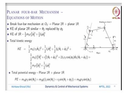
So, we have to derive the equation of motion, we break this 4-bar mechanism at  $O_3$ , so we break it here. And as a result once you break it you will have a 2R chain a serial chain and a 1R chain, very simple. We have done this earlier also when we looked at the kinematics of a 4-bar mechanism. So, the equations of motion can be very simply derived for this 2R chain and this 1R chain.
