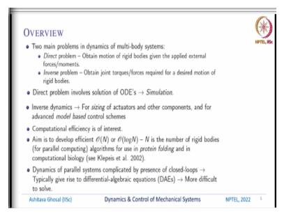
So, let us continue with overview. There are 2 main problems in dynamics of multi-body systems; the first is called the direct problem. The direct problem we obtain the motion of the rigid bodies which make up the multi-body system given the applied external forces and moments. And in the inverse problem we obtain the joint torques and forces required for a desired motion of the rigid bodies. So, what do we have?
