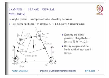
Similarly, for this closed loop simplest possible mechanism which is a 4 bar mechanism, we can derive the equations of motion. Remember, it is a 1 degree of freedom closed loop mechanism, there are 3 moving bodies 1, 2 and 3, we have only 1 actuation, so that is the torque  $\tau_1$  and it is rotating  $\theta_1$ . The other 3 angles  $\phi_1$ ,  $\phi_2$  and  $\phi_3$ , they are passive, there is only one single actuating torque.
