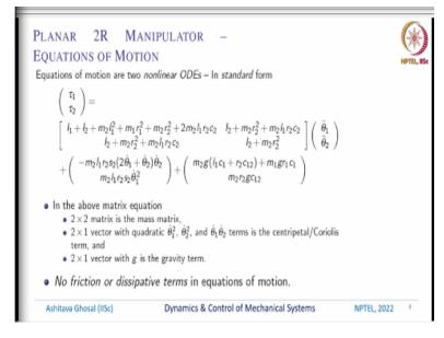
So, let us continue for the planar 2R manipulator, we can obtain the equations of motion. The equations of motion are 2 non-linear ODE's, in the standard form they are given us some  $\tau_1$ ,  $\tau_2$ = sum matrix into  $\ddot{\theta}_1$  into  $\ddot{\theta}_2$ , it is a 2 by 2 matrix plus a vector which contains  $\dot{\theta}_1$ ,  $\dot{\theta}_2$ ,  $\dot{\theta}_2^2$ , 2  $(\theta_1 + \dot{\theta}_2), \dot{\theta}_1^2$ .
