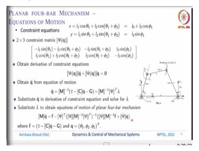
So, how do I obtain this coupling? We go back and look at the constraint equation. So, what are the constraint equations? It is  $x = l_1 \cos \theta_1 + l_2 \cos(\theta_1 + \phi_2) = l_0 + l_3 \cos \phi_1$ , this is seen earlier. y component is of that point where we are broken is  $l_1 \sin \theta_1 + l_2 \sin(\theta_1 + \phi_2) = l_3 \sin \phi_1$ . And we can differentiate these equations and then we get this 2 by 3 constraint matrix.
