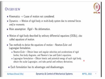
So, in overview: In kinematics we do not consider the cause of the motion; we look at the geometry of motion basically. In dynamics the motion of a rigid body or a multi-body system due to external forces and or movements are considered. The main assumption is that the multi-body system contains only rigid bodies; there is no deformation in the bodies which make up the multi-body system.
