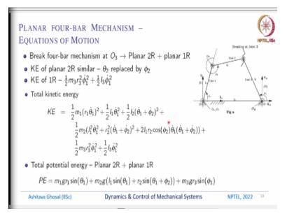
So, we break this four-bar at  $O_3$ , so we have a plana 2R and a planar 1R system. 2R means 2 links connected by 2 rotary joints and this other one is a planar 1R which is nothing like but similar to a pendulum. So, the kinetic energy of this 2R is very similar to what we have derived earlier, all we need to do is replace  $\theta_2$  by  $\phi_2$ . So, in the place of the planar 2R we have  $\theta_1 \theta_2$ , now we have  $\theta_1$  and  $\phi_2$ .
