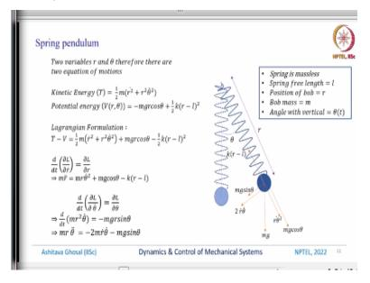
This example is a modification of a simple pendulum, the modification is as follows. So, we have a bob which is connected not by a wire or a rope but with the spring. So, as you can see there is gravity acting downwards, so this bob can move in some path which is sort of like an arc of a circle but it can also go up and down. So, there are 2 variables r and  $\theta$  which need to be used to describe the motion of this bob.
