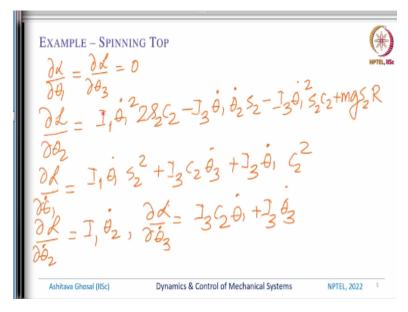
So, let us compute all these terms in the partial derivatives and ordinary derivatives. So,  $\frac{\partial L}{\partial \theta_1}$  and  $\frac{\partial L}{\partial \theta_3}$  is 0, there is no theta, only the Lagrangian is function of  $\theta_2$ . The Lagrangian with respect to  $\theta_2$ ,  $\frac{\partial L}{\partial \theta_2}$ , you will get all these terms. So, you will get  $I_1 \dot{\theta}_1^2 2 s_2 c_2 - I_3 (\theta_1) \dot{\theta}_2 s_2 - I_3 (\theta_2) s_2 c_2 + mgs_2 R$ .
