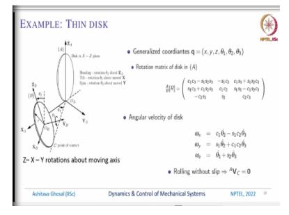
Let us take one more example. This is an interesting example of a thin disk which is rolling on the ground with no slip, this we have discussed earlier this is an example of non-holonomic constraint. So, we have this disc initially in the X-Z plane, so there is a heading angle which is  $\theta_1$ which is rotation about the Z-axis. Then there is a tilt rotation  $\theta_2$  above the moved X-axis and then there is a spin which is the rotation  $\theta_3$  about the moved Y axis.
