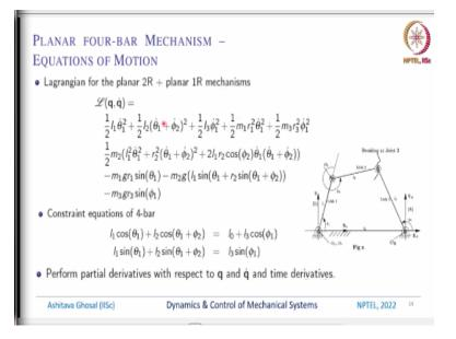
The Lagrangian for the planar 2 R + the planar 1 R mechanism is nothing but sum of all these kinetic energies. So, it is  $\frac{1}{2}I_1\dot{\theta_1}^2 + \frac{1}{2}I_2(\dot{\theta_1} + \dot{\phi_1})^2 + \frac{1}{2}I_3\dot{\phi_1}^2$ . So, this is coming from the 1R chain or from the simple pendulum, these 2 are coming from the 2R chain. And then we have of course  $\frac{1}{2}m_1r_1\dot{\theta_1}^2 + \frac{1}{2}m_3r_3\dot{\phi_1}^2$ , this is coming from that 1R chain.
