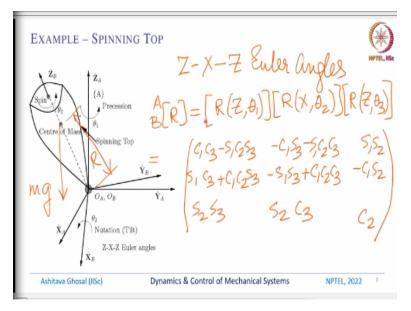
The first example is a very classical example we are going to consider the spinning top, we have already considered the scene what a spinning top does when it is not subjected to an external force earlier on. But now we will look at a spinning top when there is a mg force which is acting at the center of mass here. So, if you recollect the spinning top can be described by Z-X-Z Euler angles. So, what is Z-X-Z Euler angles?
