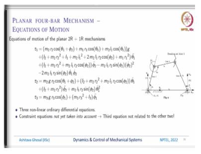
So, the equation of motion for the planar 2R and 1R mechanism can be written down. We just collect all the terms which contains  $\ddot{\theta_1}$  which is this, collect all the terms which contains gravity, which is this, collect all the coriolis and centripetal term which are these, this one and this one and collect all the terms which contains  $\ddot{\phi_2}$ . So, this is from the 2R chain.
