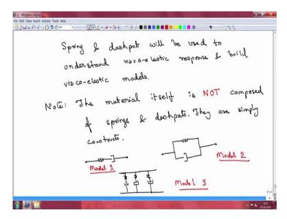
So, spring and dashpot will be used to understand viscoelastic response and build viscoelastic models. Now, we must clarify here that the material itself is not made of the spring and dashpot, they are just imaginary constructs that we can use to model viscoelastic response. So, please note the material itself is, I will just use red to highlight, is not composed of springs and dashpots they are simply constructs.
