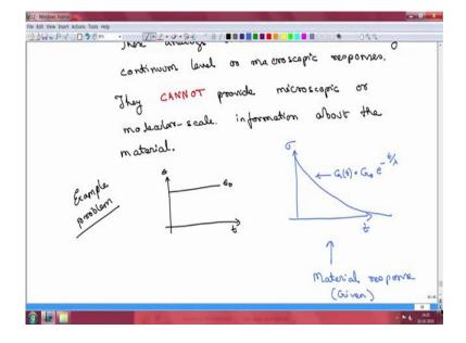
The material response is already shown to you, and this has given to a strep strain test.
