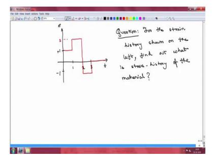
Now, the question is that was being posed for you is that this same material is now going to be subjected to strain where the strain is for a duration of 1 time time delta t equal to 1, the strain is 1, thereafter it increases to a value of 2. So, this value here is 2 when it remains at 2 till t equal to 2 after which decreases to a value of minus 1 and remains at a level of minus 1 till delta t of 1 and at time t equal to 3 it becomes 0.
