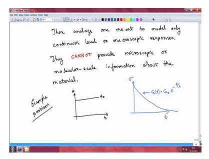
So, before we sort of end our discussion on analogs we will just note that these analogs are meant to model only continuum level or macroscopic big responses. They cannot model or they do not have any information about the microscopic details of the material, so they cannot provide and maybe here and just they cannot, they cannot provide microscopic or molecular scale information about the material.
