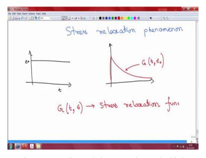
So, for the stress you what you are going to do is you need to apply this known amount of strain to the system, this curve which we have labeled separately as ABC so now you see why you had broken up the curve in different parts. This curve is again a function of time, it is again a function of the imposed strain, right. So this curve is also called the stress relaxation function.
