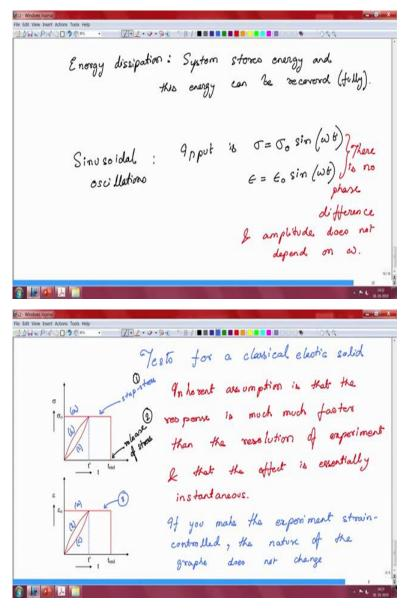
So, with regards to energy dissipation. We have seen that just go back that when you apply a known amount of stress the system goes to a certain amount, registers a certain strain and this strain holds for as long as you want infinite. That is just our simplification obviously that cannot be true but, for the theoretical or a for a theoretical prospective, the idea of a classical elastic solid is that, it can hold that amount of strain for an infinite amount of time.
